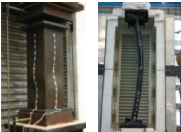
Ofenversuche. Tests zum Querschnitts- (links) und Knickwiderstand (rechts). Structural electric furnace tests. Cross-sectional capacity test (left) and column strength test (right).
