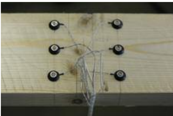
Experimentelle Untersuchung lokaler Materialeigenschaften an Holzbrettern. Experimental analysis of local material properties of timber boards.
