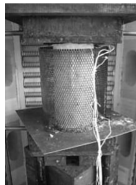
Betonprobe im Brandofen. Concrete specimen in the furnace.
