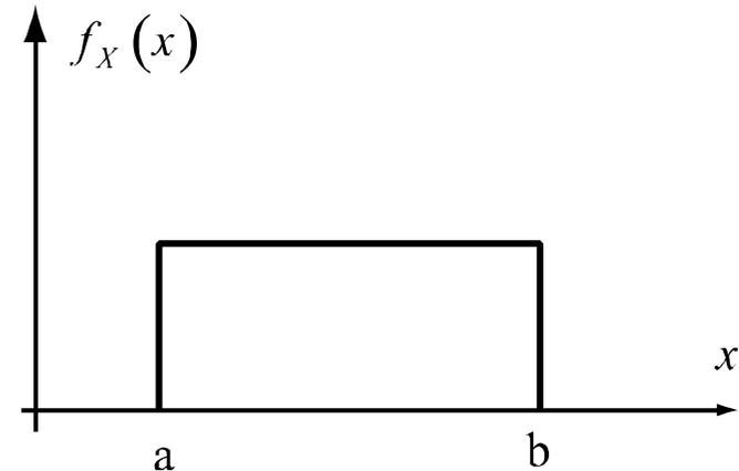
$$F_X(x; a, b) = \begin{cases} 0, & x < a \\ \int_a^x f_X(y; a, b) dy = \int_a^x \frac{1}{b-a} dy = \frac{(x-a)}{(b-a)}, & a \leq x \leq b \\ 1, & x > b \end{cases}$$
