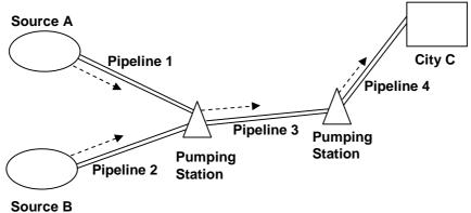
The failure of a pipeline will lead to a shortage of water in the city. If events  $E_1$ ,  $E_2$ ,  $E_3$  and  $E_4$  denote the failure of pipelines 1, 2, 3 and 4 respectively, the event that there is no shortage of water in city *C* can be written in the following way(s):
