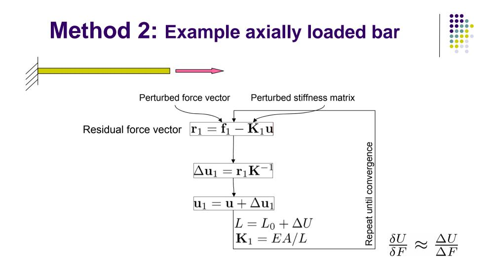
Original stiffness is used in every iteration to calculate the perturbed displacements. A new residual vector is defined and predictor-corrector sequence is repeated until convergence of the perturbed solution
