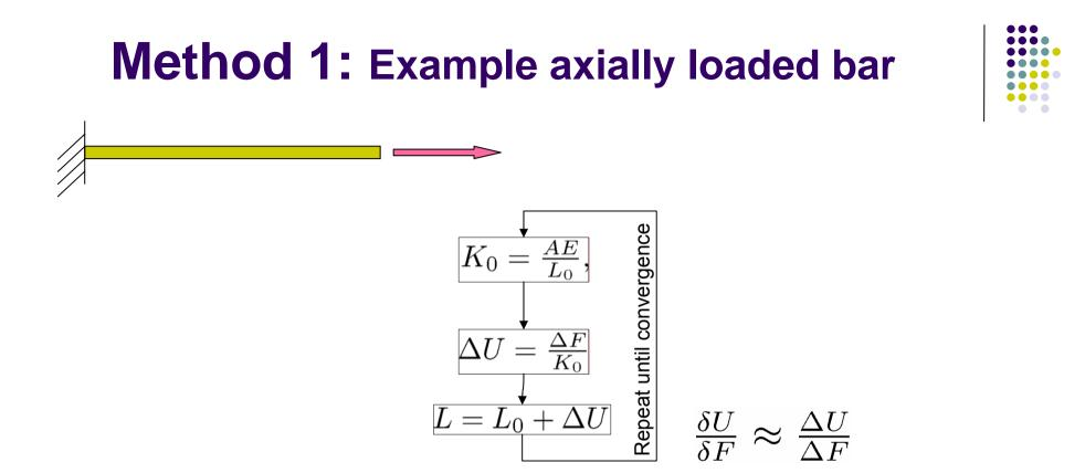
For a small variation in the load, an iterative solution for the response is computed
