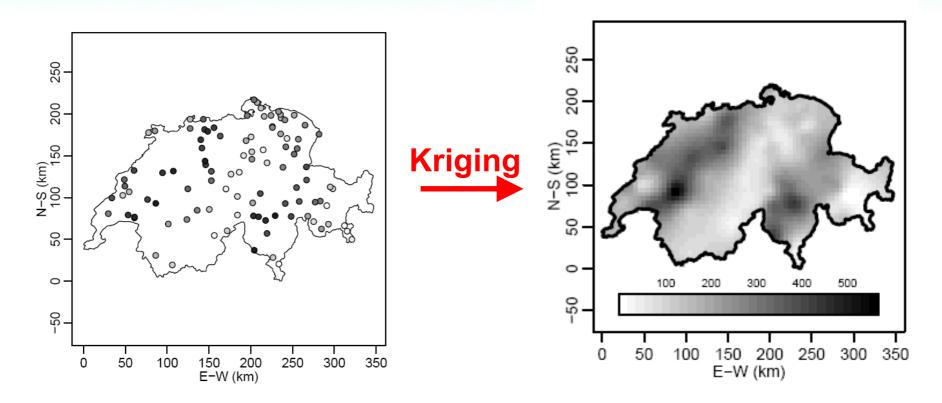
Transformed gaussian model (Box-Cox transformed data) with Mathérn correlation structure.
